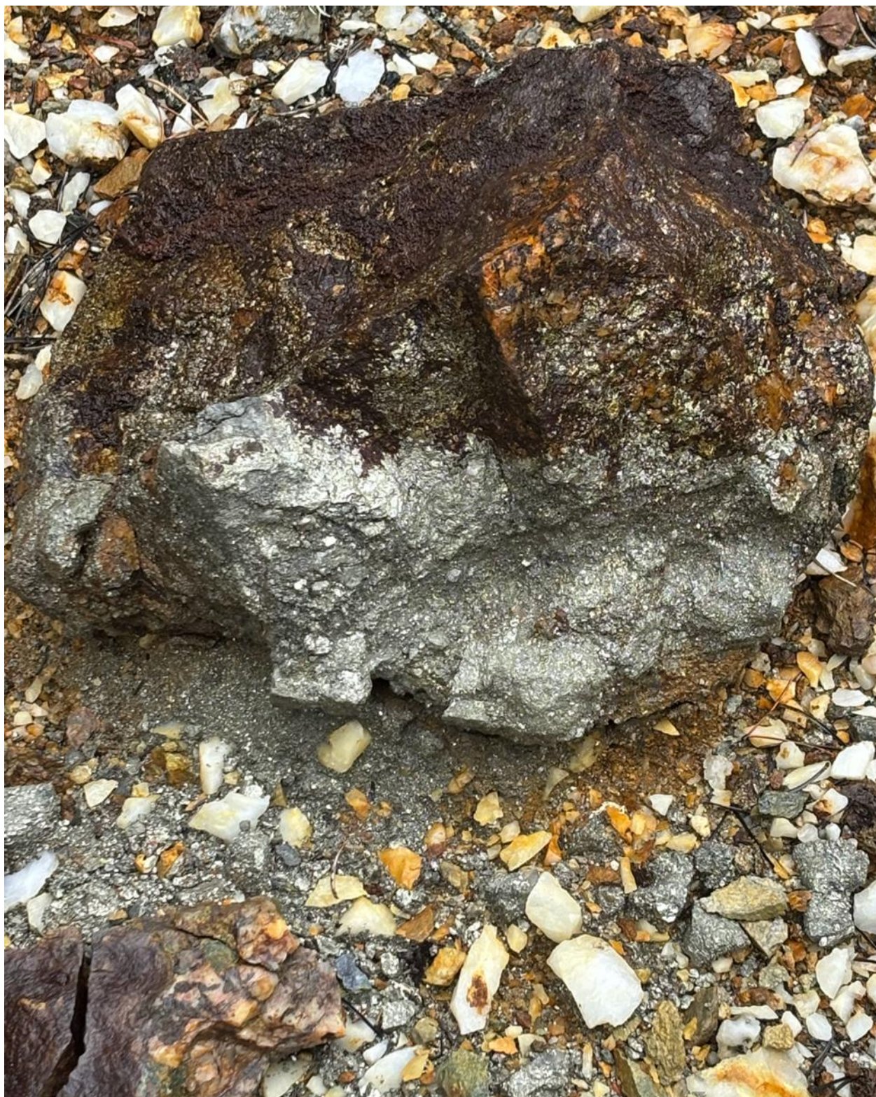
Heavily Mineralized 4 ft Wide Boulder from Quartz Vein Near the Shaft
