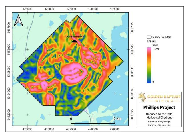
There are weakly magnetic N-S trending linear anomalies located in the middle of the survey area. Of importance is that these are overprinted by the stronger magnetic anomalies seen in the figures, implying that they are from a previous deformation event.
